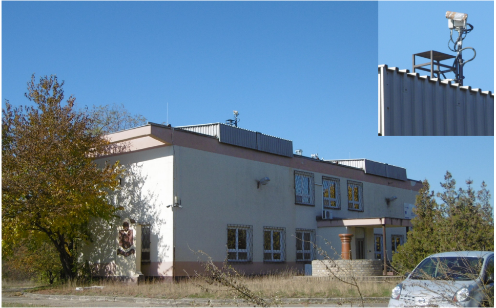
Fig. 2: Baja Astronomical Observatory with the TLE camera on the roof (zoomed-in image is on the inset).
