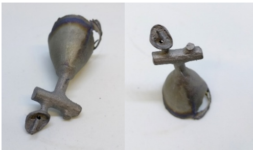
Fig. 6: Workpiece with argon gas generated casting cavities
