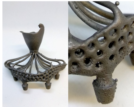
Fig. 8: A cortically supported individual implant with small bubbles present
