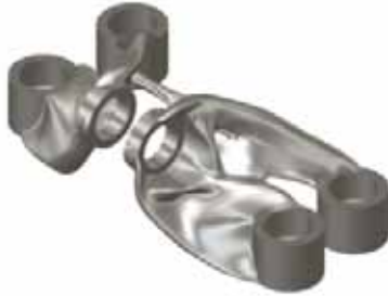
Figure 11.: Generated design unrestricted manufacturing method
