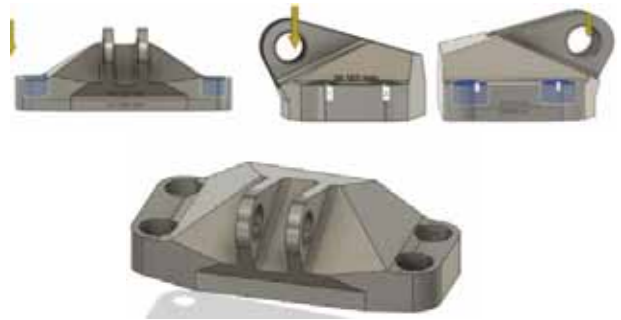
Figure 5.: Starting the shape of the GE bracket with the main dimensions
