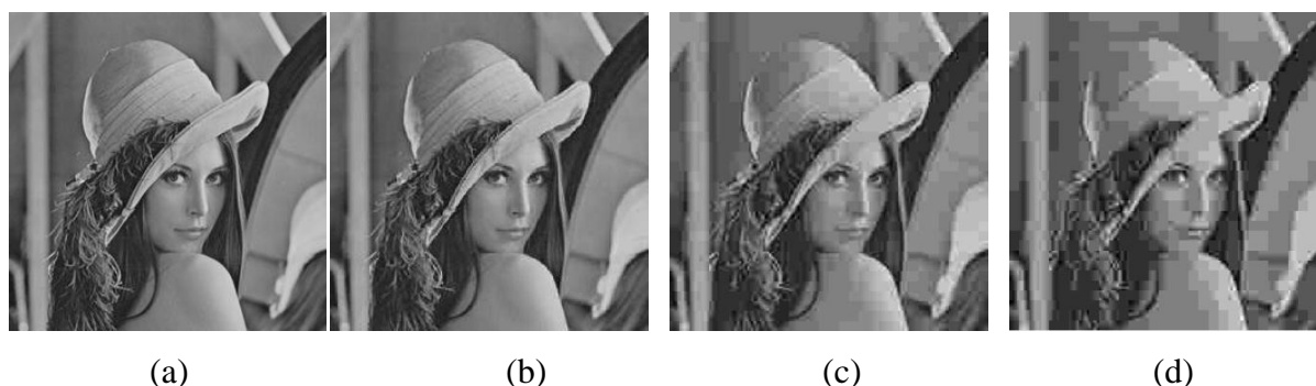
Fig. 1. Test image Lena with different compression ratios. (a) Original Lena image, Size: 64kB, bitrate: 8bpp, (b) Lena test image compressed with compression ratio 11, Size: 5.8kB, bitrate: 0.73bpp, (c) Lena test image compressed with compression ratio 30, Size: 2.1kB, bitrate: 0.27bpp, (d) test image Lena compressed with compression ratio 46. Size: 1.4kB, bitrate: 0.17bpp.
