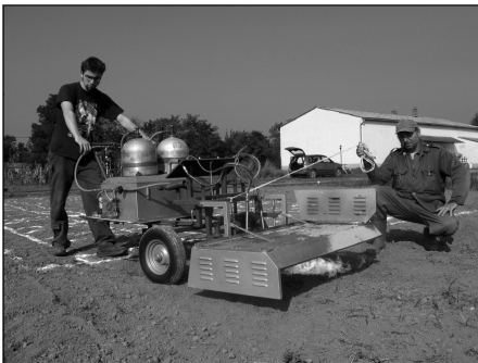
Figure 1. Manual, wheel-barrowed weed flamer
