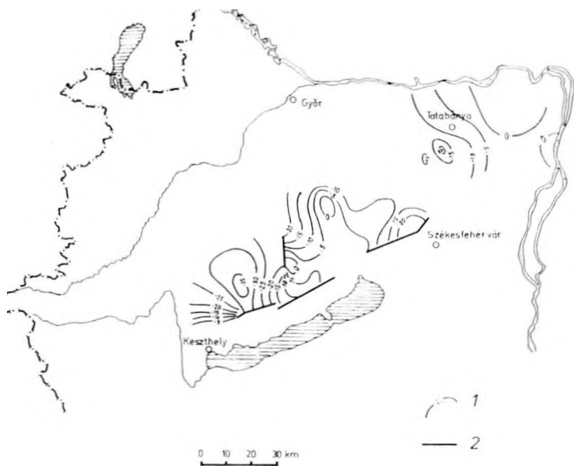
Fig. 4. Map of difference of karst water level. 1. Difference of water level. 2. Impermeable zones.
