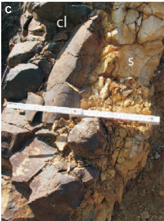
Baked silt/sand (s) at the contact of basanitic body (cl) and host sediment (photo courtesy of Manuella Kramer)
