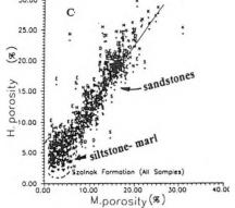
Fig. 5. Relationships between helium porosity and mercury porosity. A—sandstones; B—silt-stone-marls; C—all samples
