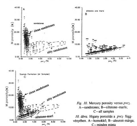
and siltstone-marls have a range of pvc<sub>2</sub> % from 1.0 up to 10.0 of total pore volume. A linear regression line equation has been calculated for siltstone-marl facies, this being:
