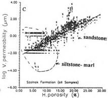
Fig. 7. Helium porosity versus vertical permeability. A—sandstones; B—siltstone-marls; C—all samples
