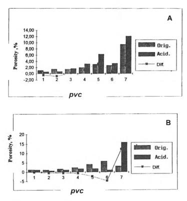
Fig. 17. Effect of calcite cement on both porosity and permeability before and after acidification (Szarvas area). A—sandstone reservoir type-1; B—sandstone reservoir type-2
