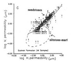
Fig. 8. Horizontal permeability versus vertical permeability. A—sandstones; B—silt-stone-marls; C—all samples
