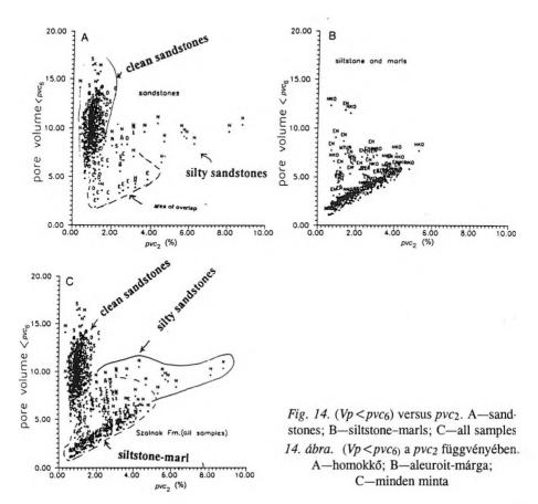
By using these relations one can determine the effective pore radius, which is difficult in measurements as well as being expensive, from the routine porosity data of the Szolnok Formation.
