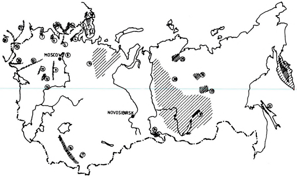
Fig. 24. Scheme of crustal conductivity anomalies [according to ZHAMALETIDINOV]. Anomalies: 1—Pechenga; 2—Keivskaya; 3—Tiksheozersko-Belomorskaya; 4—Onega; 5—Ladoga; 5 a —Ladoga-Botnicheskaya; 5 b —Ladoga-Wennem; 6—Chudskaya; 7—Baltic; 8—Vologda; 9—Moscow-Tambov; 10—Kirovograd; 11—Kursk; 12—Voroncovo; 13—Carpathian; 14—Timan-Pechora; 15—Ilovlya; 16—Tien-Shan; 17—Fergana; 18—Anabar; 19—Bodaibo; 20—Voi-Siberian; 21—Kamchatka; 22—North Sakhalin; 23—Vilyuisk; 24—Minusa; 25—Khatanga; 26—Izmail-Poltava; 27—North German; 28—Pannonian
