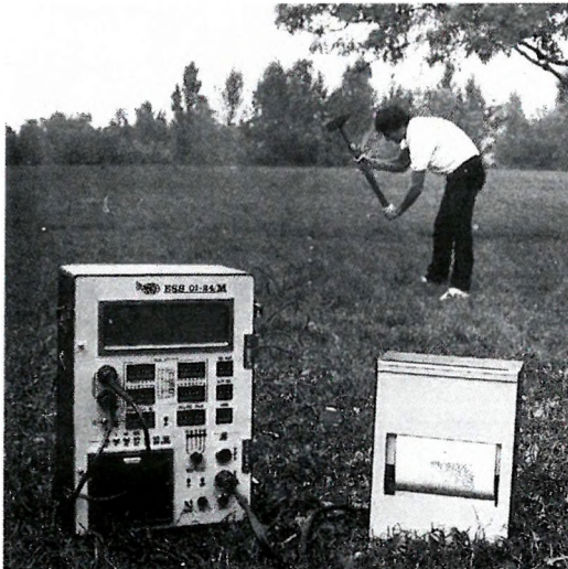
Field work with ELGI's 24-channel portable seismograph
