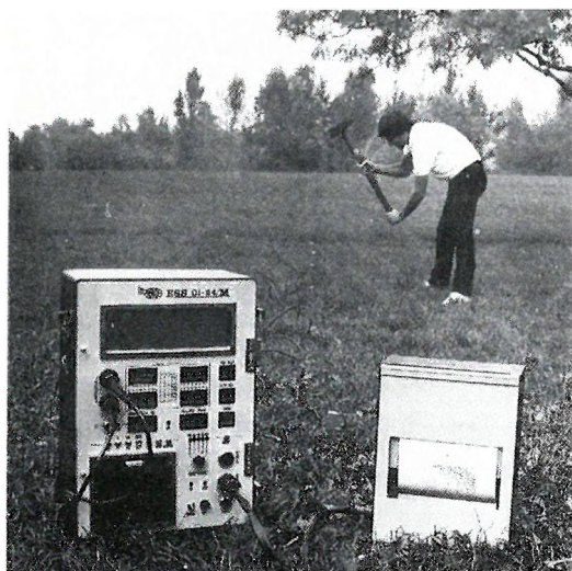
Field work with ELGI's 24-channel portable seismograph
