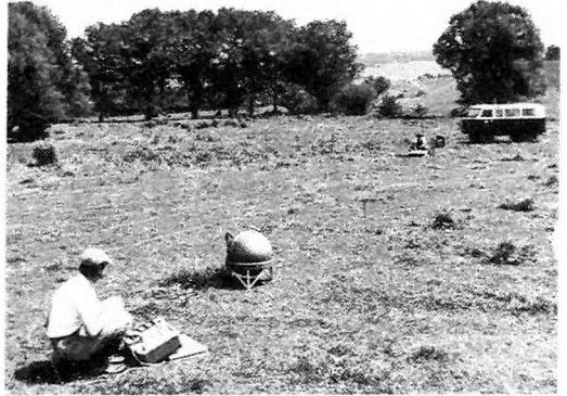
The Maxi-Probe electromagnetic sounding and mapping system – produced under licence by Geoprobe Ltd. Canada – is an ideal tool for shallow depths, especially in areas where seismic results are poor or unobtainable
