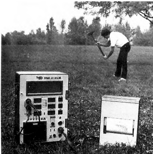
Field work with ELGI's 24 channel portable seismograph
