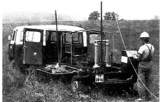
ELGI has a vast experience in solving problems of environmental protection such as control of surface waters, reservoir construction, industrial and communal waste disposal, protection of surface and ground water etc. ELGI's penetrolgger provides in-situ information – up to a maximum depth of 30 m – on the strength, sand/shale ratio and density without costly drilling.
