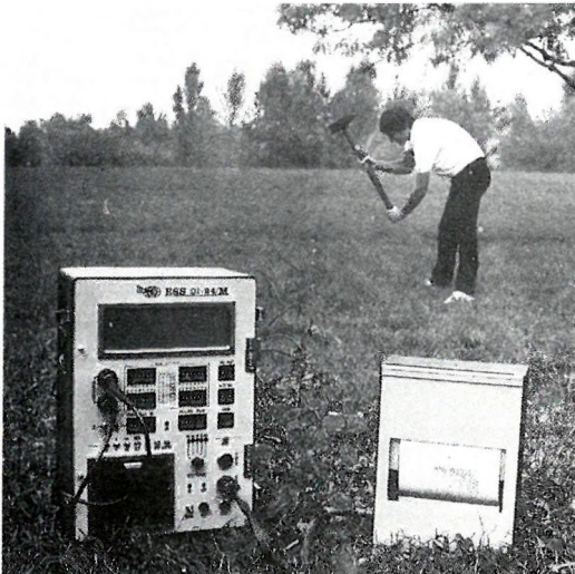
Field work with ELGI's 24-channel portable seismograph
