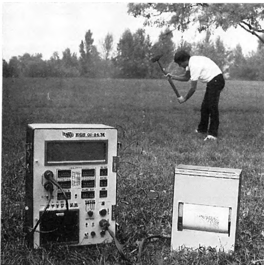
Field work with ELGI's 24-channel portable seismograph
