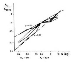
Fig. 1. Total amplitude of seismic waves as a function of charge quantity, Q [after Levyant 1964].  $H_a$  - charge depth;  $h_a$  - thickness of low-velocity layer
