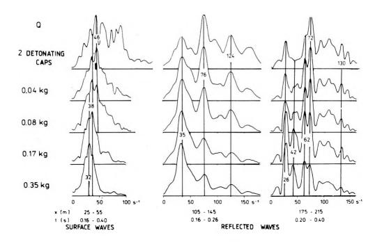
Fig. 2. Amplitude-frequency spectra for variations of charge quantity, Q, and for different distances x from the shot point and different time intervals  $\Delta t$ . Charge depth: 15 m, closely below low-velocity layer
