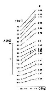
Fig. 6. Spectral amplitudes of reflected waves as a function of charge quantity for determining exponent p (for data, see Fig. 2, centre column)
