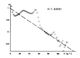
Fig. 9. Exponent p as a function of frequency, determined from spectral division for two charge quantities  $(Q_2 = 0.17 \text{ kg}, Q_1 = 0.04 \text{ kg})$
