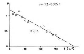
Fig. 7. Exponent p as a function of frequency (values from Fig. 6)
