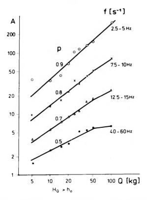
Fig. 5. Amplitudes of seismic waves as a function of charge quantity, Q, for different frequency intervals [after Molottova 1964].  $H_{\rm O}$  - charge depth;  $h_{\rm o}$  - thickness of low-velocity layer
