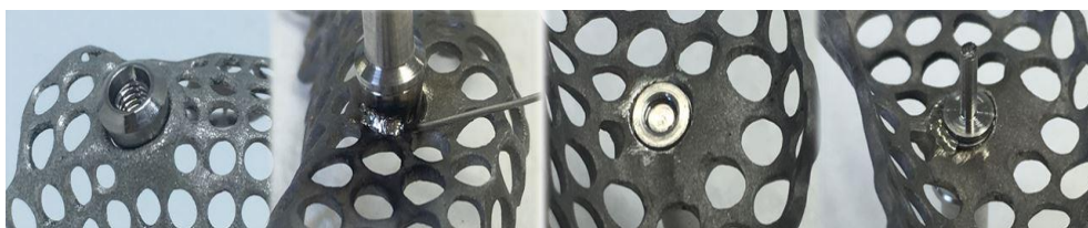
Fig.22 Welding process of positioned threaded sleeve
