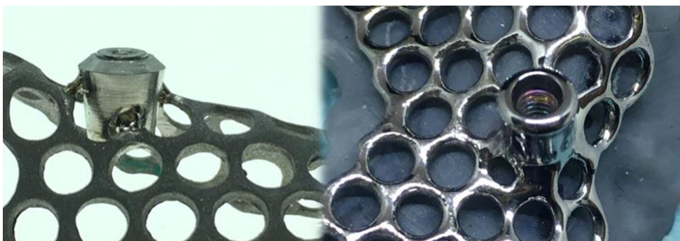
Fig.14 Welded pillar structure
