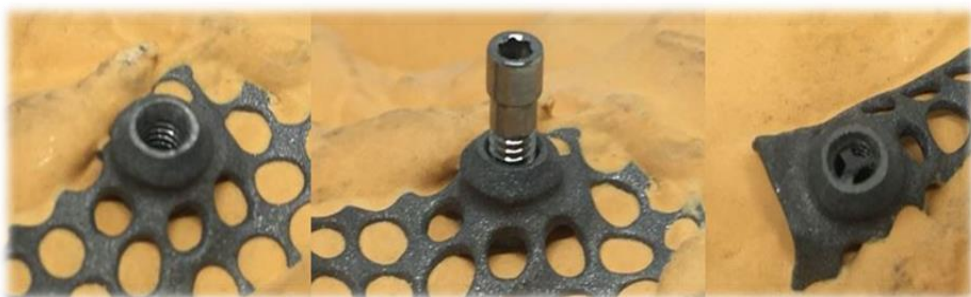
Fig.21 Trial thread tapping in 3D-printed titanium baseplate
