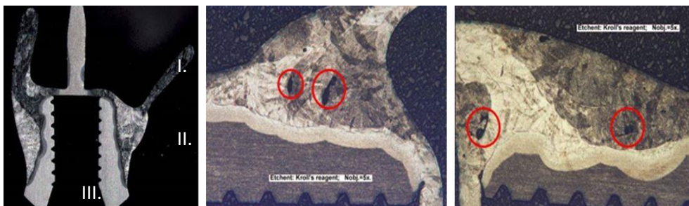
Fig.24 Metallographic section of the welded joint
