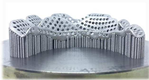
Fig.19 3D-printed Grade 23 titanium baseplate
