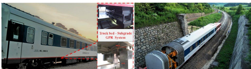
Figure 2 Subgrade inspection device
