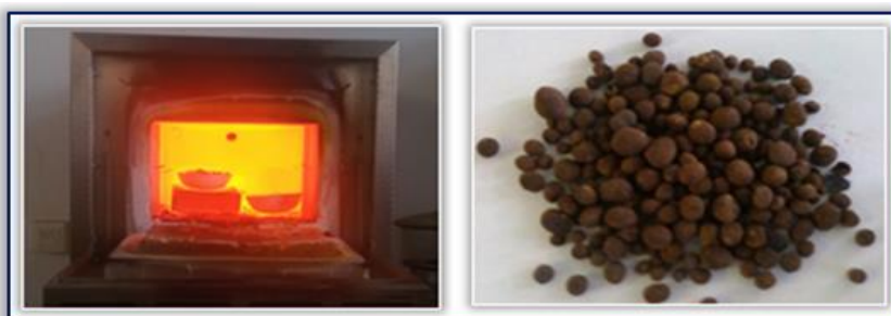
Figure 6 Hardening of the pellets [12, 24]
