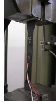
Figure 20 Test specimen in the tension test machine
