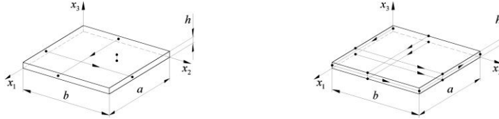
Figure 14 Connecting the nodes for ensuring the periodicity
