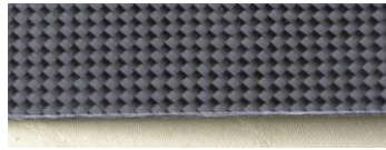
Figure 4 Eight-layer textile composite plate
