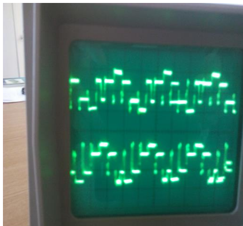
Figure 17 The output voltages - Phases U_R and U_S
