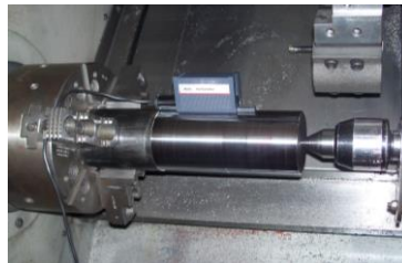
d) Surface roughness measurement
