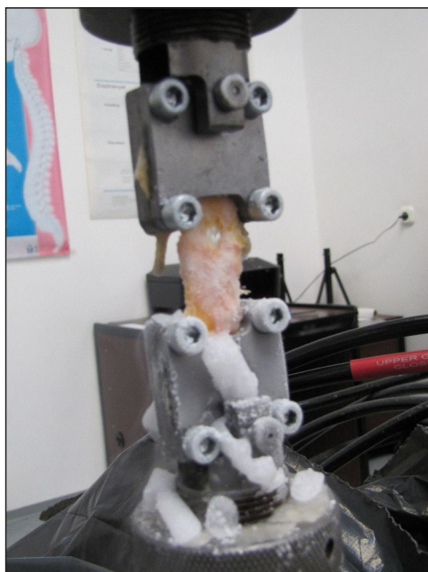
Figure 1. Test setup of the fatigue test
