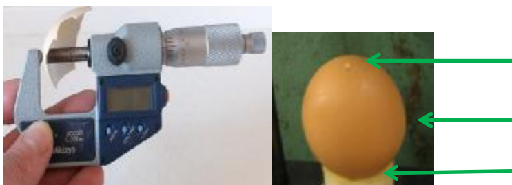
Photo 2: Determination of thickness of egg shell
